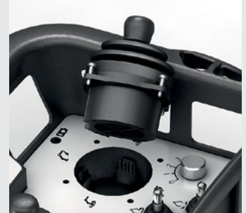
SMJ technology SMJ joysticks (1- and 2-axis) are integrated in the console housing with positive locking without housing openings. Joysticks can therefore be changed directly on site without risk of contamination if there is a fault.
