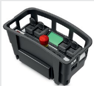
Nano-L SMJ A1/4 with display Modular system design Example with four SMJ joysticks, 1-axis Data feedback on monochrome display Medium-size console (Width 248 x Depth 140 x Height 118)
