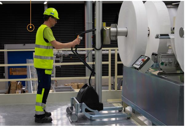
At SCA in Sweden, several lifting trolleys are used to pick up reels from pallets and transport them to machines. The reels are easily positioned and mounted on the machines. All with the ergonomic help of TAWI lifters.
