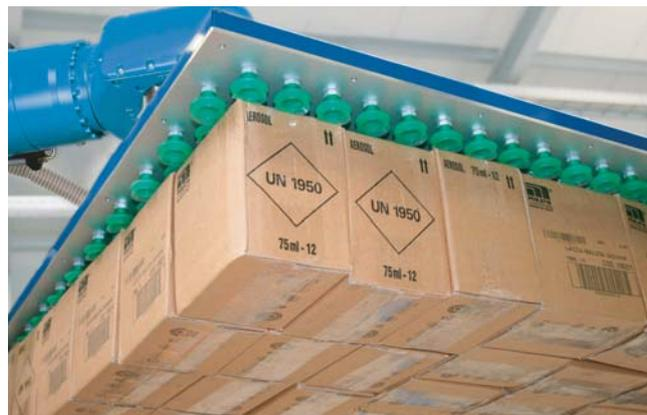
SPZ Packaging | 包装纸箱、饮料托盘等的整层码垛和拆垛
