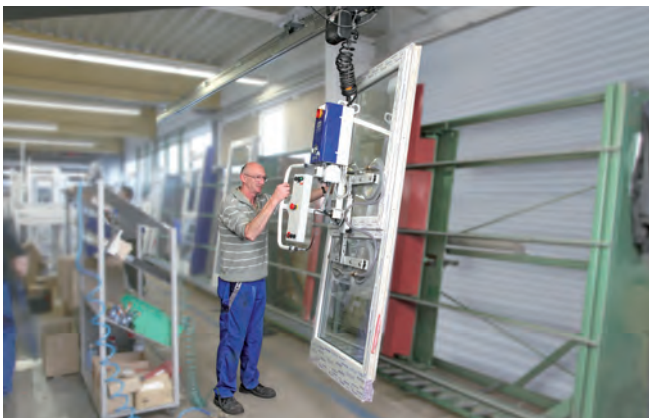
Vacuum lifting device VacuMaster Window Comfort being used to handle a multi frame window
