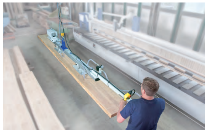
Vacuum lifting device VacuMaster VHB for unplanned boards and planks
