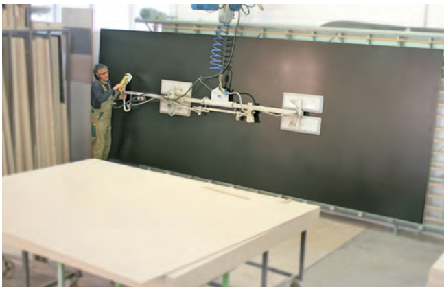
Vacuum lifting device VacuMaster HHVM being used to load a vertical saw
