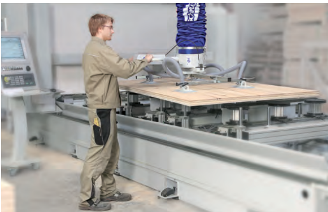
Vacuum tube lifter JumboErgo being used to load a CNC machining center
