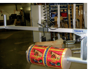
An outbalanced boom for reel lifting.
