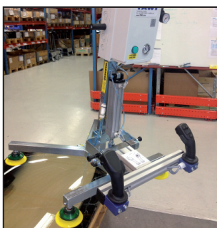
Lifting glass car wind- shields using dual joystick control
